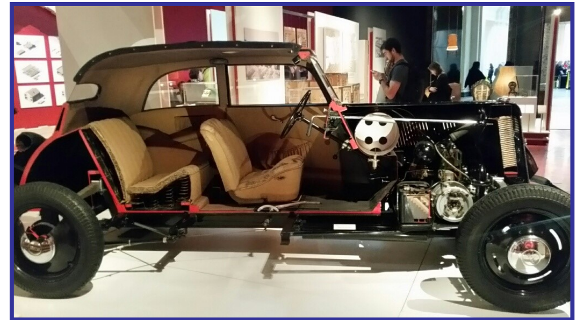
Cross section of an old automobile illustrating the extensive use of Plywood
